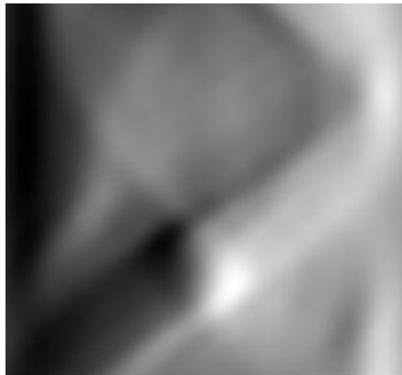
Figure 16: Sinogram filtered by the Hilbert filter.
