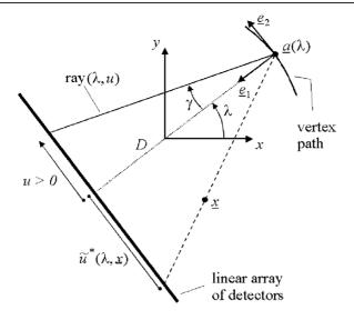
Figure 7. Fan-beam geometry with equally spaced collinear detectors.
