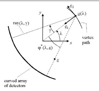
Figure 5. Fan-beam geometry with equi-angular rays.
