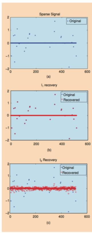
[FIG2] (a) A sparse real valued signal and (b) its reconstruction from 60 (complex valued) Fourier coefficients by  $\ell_1$ minimization. The reconstruction is exact. (c) The minimum energy reconstruction obtained by substituting the  $\ell_1$  norm with the  $\ell_2$  norm;  $\ell_1$  and  $\ell_2$  give wildly different answers. The  $\ell_2$  solution does not provide a reasonable approximation to the original signal.
